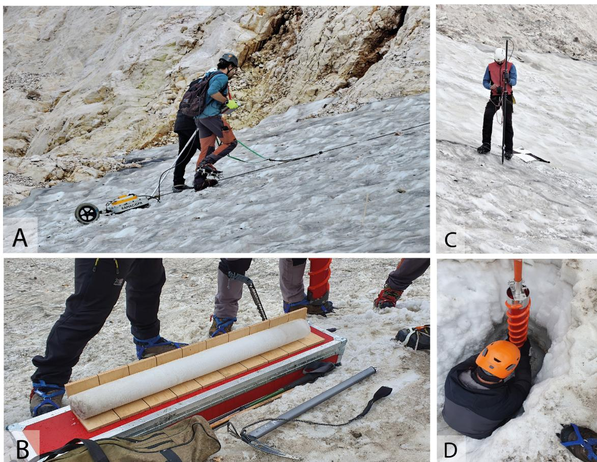
**Figure 3** - Work activities on the Triglav Glacier in 2022: (A) Ground penetrating radar measurements, (B) ice core sampling, (C) GNSS measurements, (D) drilling of the ice core.
